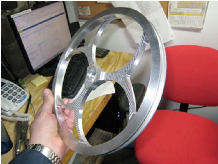
Through answering online bids and sending clients CAD files straight into streamlined CNC milling, Tosa Tool creates one-offs of mechanical parts in a few hours.
