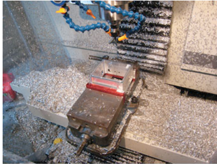
The Tormach PCNC 1100 tips the scales at a little over 1130 lb (512 kg) with a 1.5-hp (1.1-kW) spindle and can handle a variety of workpieces to 500 lb (226 kg).
