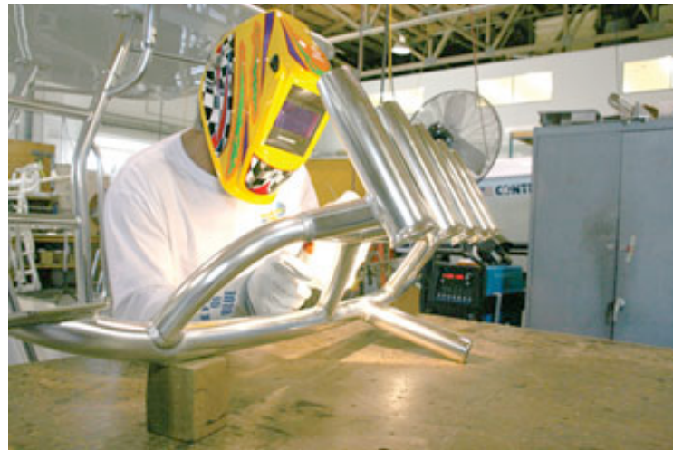
The Miller Dynasty 350 AC/DC TIG welder allows Bruce Saad, Birdsall fabrication manager, to weld the anodized aluminum in one pass instead of two.
